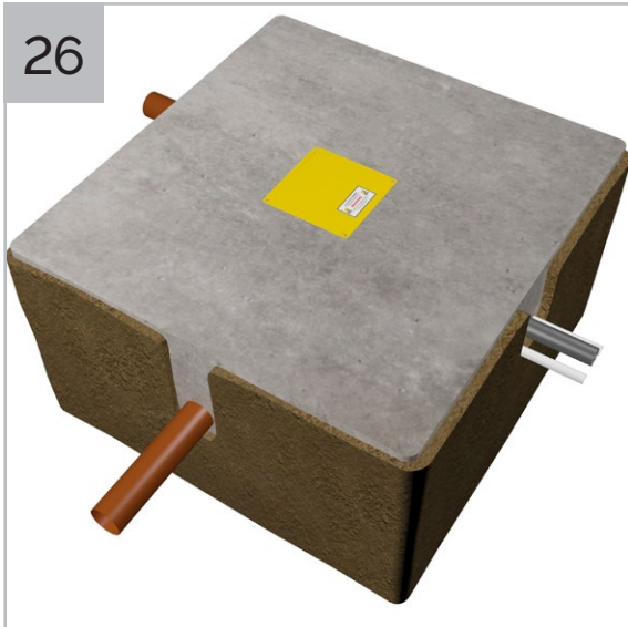
Allow concrete to cure.
