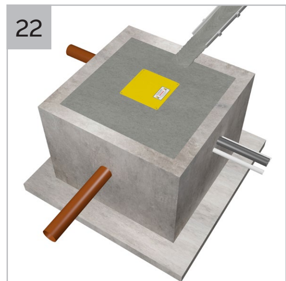
22 Fill void between RC box and chamber with concrete (we recommend use of C35 grade/PAV2 as a minimum) or as per the structural engineer's details.
