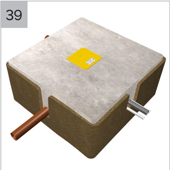
Re-fit temporary site cover to protect the pump station.
