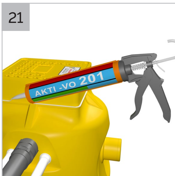
21 Once chamber has been filled with water, apply Delta AKTI-VO 201 (swellable mastic) to the entire external lip locator of chamber.
