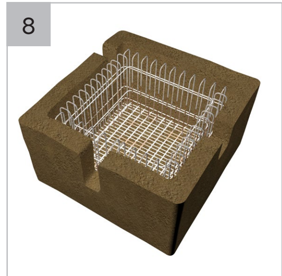
Install re-bar as per structural engineer's details.
